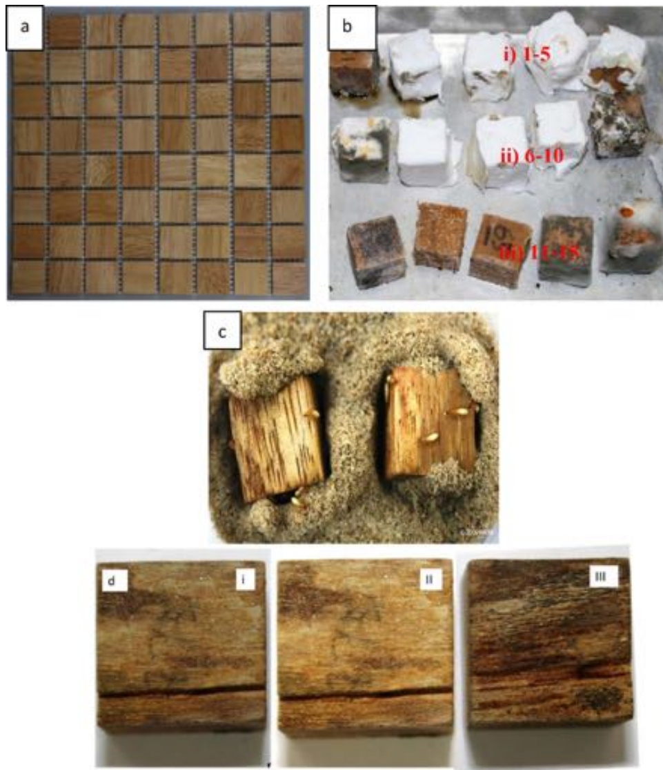
Fig. 6. (a) Rubberwood before coated with pAam-g-S coating while (b) Coated rubberwood affected by white rot fungi P Sanguineus with various ratios pAam: starch i) 2:1, ii) 1:2, and iii) 3:5. (c) Coated rubberwood attacked by termites C. Curvignathus while (d) Various ratios of coated rubberwood affected by C. Curvignathus with pAam: starch i) 2:1, ii) 1:2, and iii) 3:5.
